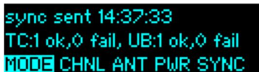
Selecting **SYNC** opens the screen for sending a sync command to all ACN-TL or ACL 204 in reach which are on the same channel and in JAM mode. Syncing is only possible from a device that has a valid time code (jammed or set manually), signaled by green flashing LED.
