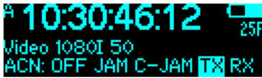
**TX** is a wireless transmission of external time code present on the Lemo/TC input. This is intended for transmitting a record-run time code to another ACN-TL or ACL 204 which is in **RX** mode.
