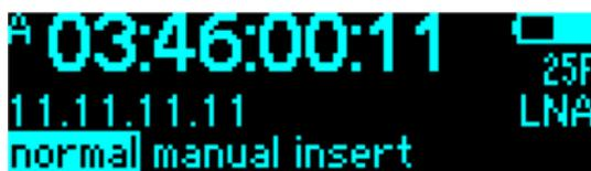
**manual**: the user bits are not being overwritten by external time code. This mode is to be used if you want a custom entry, like date and camera Id for instance.
