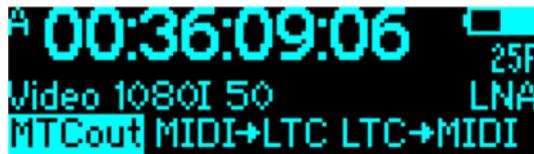
**MTCout:** this is the default mode. The ACL 204 always puts out MTC, unless the USB port is set to COM (see SYS > Config > USB).
