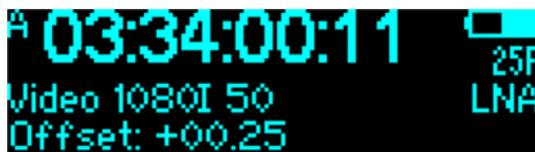
An offset can be entered between the jammed time code and the time code on the output of the ACL 204. Use this to compensate the processing delay that some file base cameras produce.
