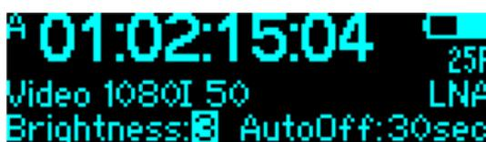
Adjust display **brightness** from 1 to 10 toggling the config switch left/right. Push in to select value.
