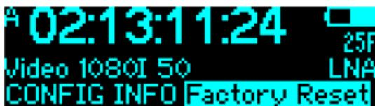
This restores factory defaults: Sync is off, TC is 25 fps, ACN is off, display brightness at 3, display auto-off 30 sec., TC-offset reset, USB to MTC.
