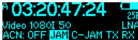
The **JAM** mode allows to send a sync command to other ACN-TL or ACL 204 devices, or receive sync command from them. This serves to remotely sync all units on the set. First, the menu asks to select the wireless channel. The **CHNL** setting allows you to select between 16 network channels within the 2.4 GHz range.
