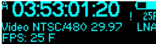
While the time code is inconsistent with the video rate, a “!” is shown next to the time code Fps indication. Select a frame rate that matches your video signal.
