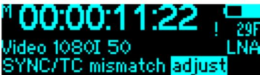
If the selected time code frame rate is incompatible to the currently set video signal type, a warning message appears:
