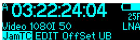
In the **GEN**enerator menu, you can edit the jam mode, edit the time and set an offset of the time code output against the jammed time.
