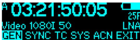
Pushing the config switch once enters the main menu screen. The main operation parameters are further displayed. In this screen, you can select the different settings by pushing the config switch. Navigate by toggling the config switch left or right.
