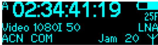
The main display is the normal operation mode. It displays the most important status information. These are the time code momentarily running, the sync signal type and rate, the time code frame rate, and various additional information:
