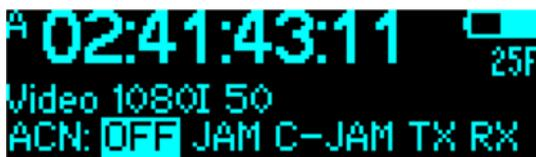
Jam – the former “BASIC” used for wireless manual jamming; C-Jam – the “continuous jam”; TX-RX for transmitting a record-run time code from external source.
