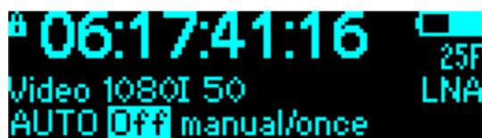
“**OFF**” – the ACL 204 does not jam to external time code. This setting is useful if you set the unit manually and not to be jammed by incoming time code.
