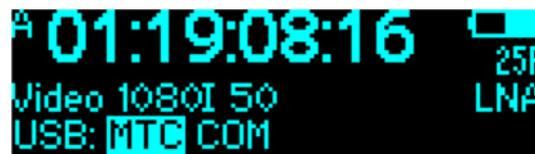
Default setting is **MTC**, the ACL 204 is recognized as Midi/Audio interface when connected to computer. Set to **COM** for updating.
