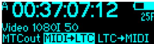
**MIDI>LTC:** MTC received through USB will be converted into LTC and put out on both Lemo sockets, pin 5.
