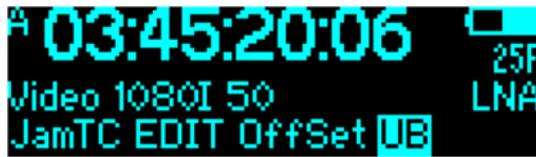
In the GEN > user bit menu, the user bits are being displayed. The user bits can be edited manually, and the jam behavior managed.
