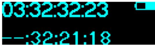
In this screen, you can edit a time code value manually. Decrease or increase by toggling left/right. Holding left/right is fast backward/ forward. Push to select.
