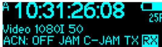
Set up channel, antenna, RF power and LNA as above in **JAM** mode.
