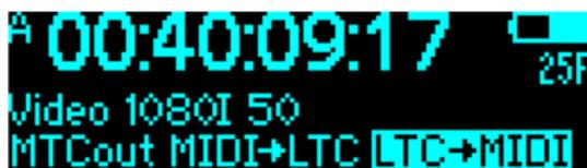
**LTC>MIDI:** LTC received on Lemo/TC pin 2 will be converted and put out as MTC via USB.
