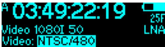
Pushing the config switch while **VIDEO** is highlighted takes you to the genlock settings. The cursor is on the signal type. Change by toggling left/right. Select by pushing the config switch.
