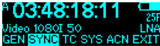
The **SYNC** menu lets you set the sync signal format, type and rate. Select the different settings by pushing the config switch. Navigate by toggling the config switch left or right.
