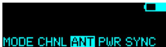
Select **internal** or **external** antenna and power the low noise amplifier **LNA** for the receiver on or off. The LNA draws power, so it is recommended only should the reception of data be insufficient without. Default setting is internal antenna, for activating the external antenna a PIN code is required.
