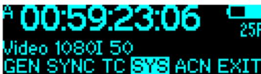
The **SYS** menu serves to configure various parameters, in this release version the display behavior and the BNC sync signal impedance are set. Push the config switch to enter.
