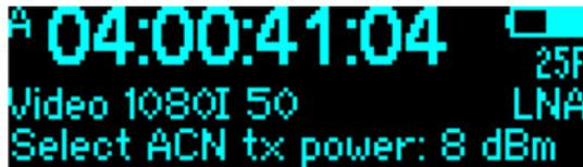
**PWR** lets you increase the output power of the transmitter. Default is 8 dBm, up to 18 dBm is possible. Again, the PIN is required.
