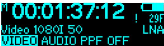
The LED will double flash and "!" is flashing next to the TC frame rate. You have no choice but to press the config switch and are automatically taken to VIDEO:
