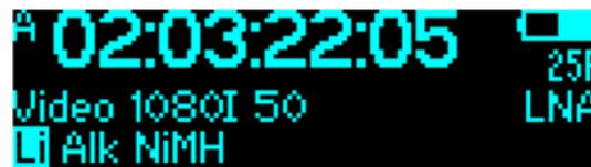
Select battery type for correct voltage readout and low battery warning / flashing.
