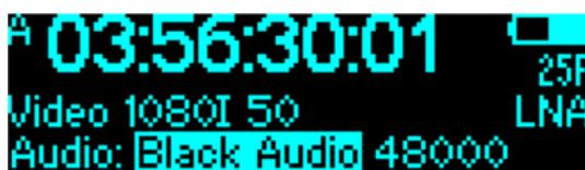
Pushing the config switch while **AUDIO** is highlighted takes you to the audio sync settings. The cursor is on the signal type selection. Change by toggling left/right.
