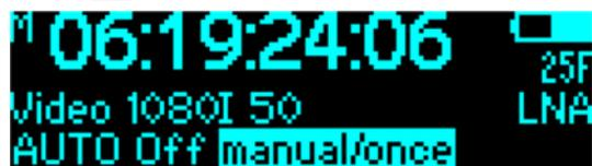
“**manual/once**” – the ACL 204 jams once to external time code, but then will not jam again but close the jam port. Once jammed, the “M” changes to
